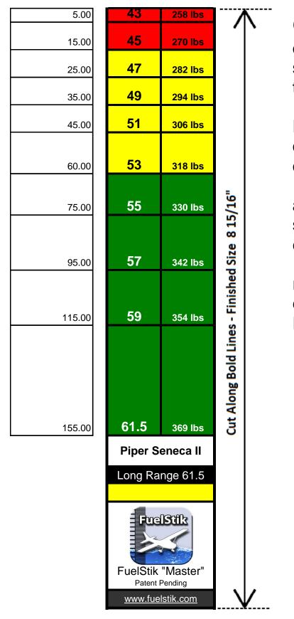
**Caution** - The operator of the FuelStik "Master" is solely responsible to assure that the correct scale is properly installed in the Float Tube and that through on-ground experience the operator has observed that the quantities shown are accurate. The FuelStik is a secondary means of estimating fuel quantity and in no way is meant to replace the fuel measuring equipment mandated by FAR's or otherwise.
